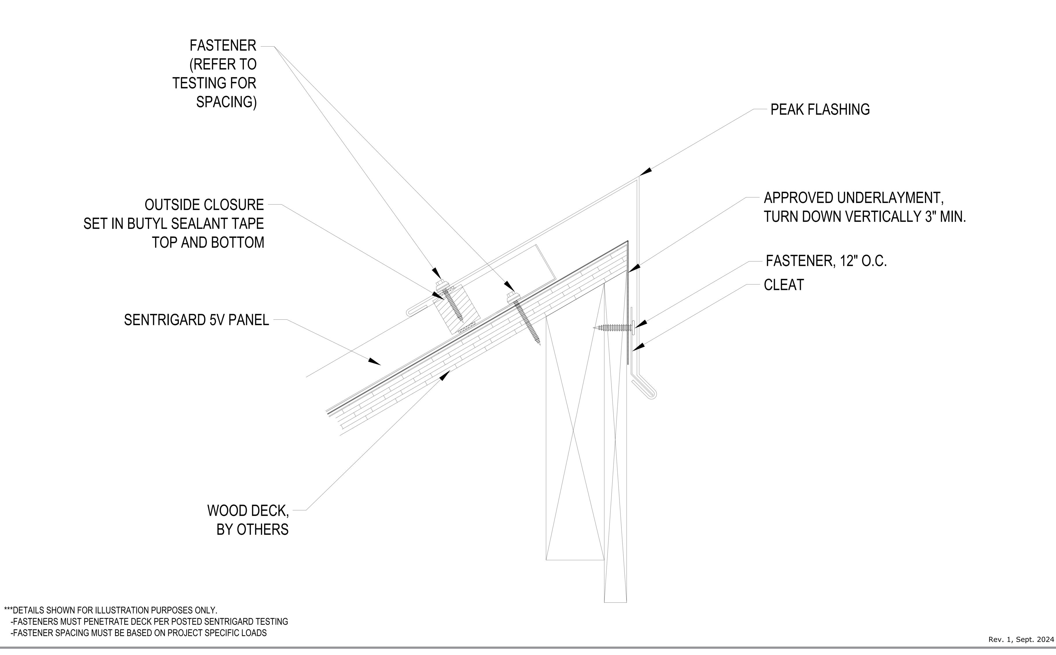
**51/**EXPOSED FASTENER METAL ROOFING SYSTEM
